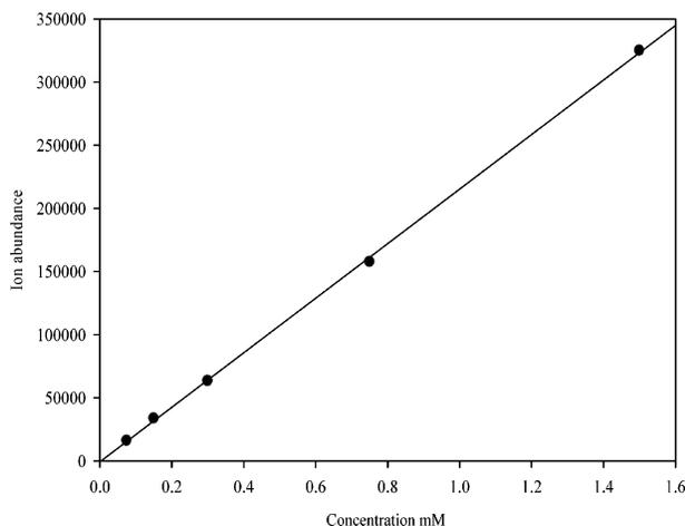
**FIGURE 3. ESI–MS response (ion abundance) to oxalic acid (*m/z* 89) in a mixed standard that included pyruvic and glyoxylic acids in the same matrix as the samples across a range of concentrations (0.075–1.5 mM compound) r<sup>2</sup> = 0.9997, y = 647 820x − 690.**
