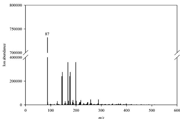
**FIGURE 5. ESI-MS spectrum of the UV degradation of pyruvic acid (no H<sub>2</sub>O<sub>2</sub> added) after 161 min. Pyruvic acid ( $m/z$  87) is present as the most abundant compound and there is a higher molecular weight cluster that is not representative of an oligomer system.**
