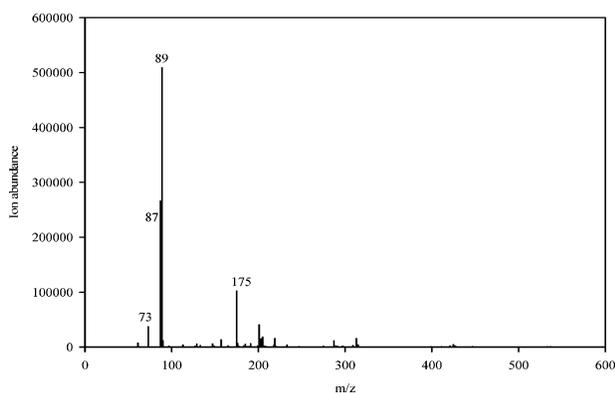
**FIGURE 2. Abundance of pyruvic acid monomer (*m/z* 87) and dimer (*m/z* 175), glyoxylic acid (*m/z* 73), and oxalic acid (*m/z* 89) in a 1.5 mM per compound mixed standard in the same matrix as the samples, detected in negative ionization mode with ESI–MS.**
