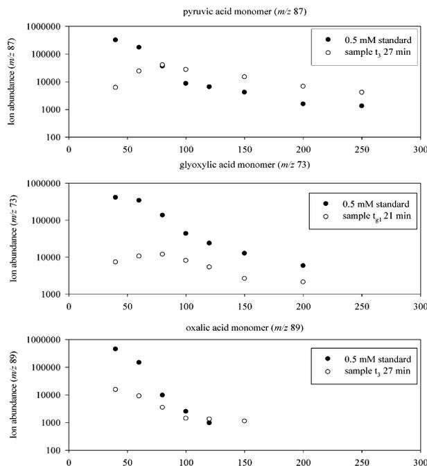
**FIGURE 6. Response (ion abundance) of pyruvic acid ( $m/z$  87), glyoxylic acid ( $m/z$  73), and oxalic acid ( $m/z$  89) to varying fragmentor voltages in a 0.5 mM mixed standard (filled circles) and time series samples (empty circles).**
