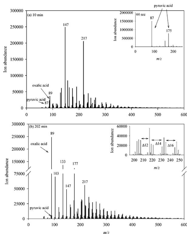
**FIGURE 4. ESI–MS spectra of time series samples from pyruvic acid UV/H<sub>2</sub>O<sub>2</sub> oxidation after (a) 10 min, and (b) 202 min. Pyruvic acid (*m/z* 87, 175) is the main compound present in a 44 s time series sample from a replicate experiment (inset a). The regular distribution of *m/z* 12, 14, 16 indicating the oligomeric system is shown for an enlarged portion of (b) in the inset. Note break in y-axis scale.**
